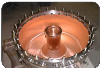
*The accelerating cavity of the Rhodotron® is immediately accessible for maintenance.*
