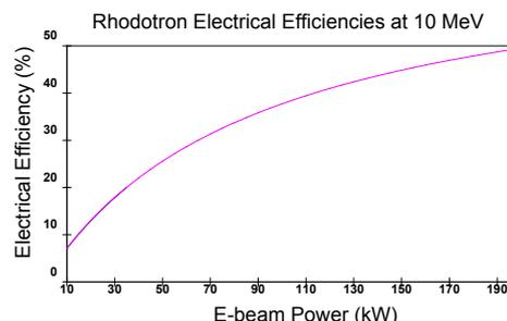
*Compared with other accelerators, the Rhodotron® is two to four times more efficient.*
